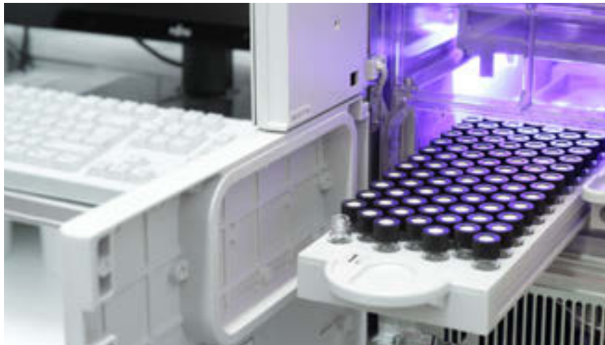
◀ Purity check of our raw materials and end products by our own HPLC (High Pressure Liquid Chromatography) / Reinheitsprüfung von Rohstoffen und Produkten mittels eigener HPLC (High Pressure Liquid Chromatography)
